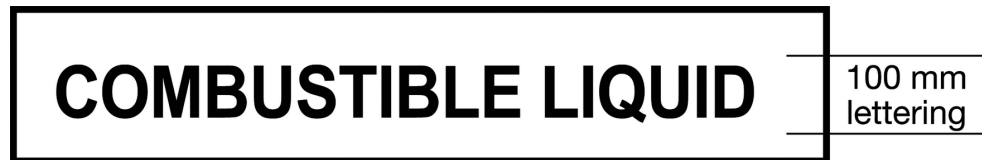
Figure 13.5 Placard for flammable liquid category 4
